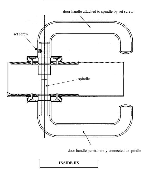
Figure 1: Schematic of typical HS door lockset
