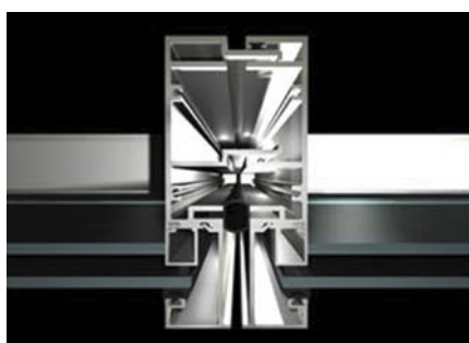
Split mullion of typical curtain wall
