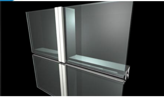
4-way joint of typical curtain wall
