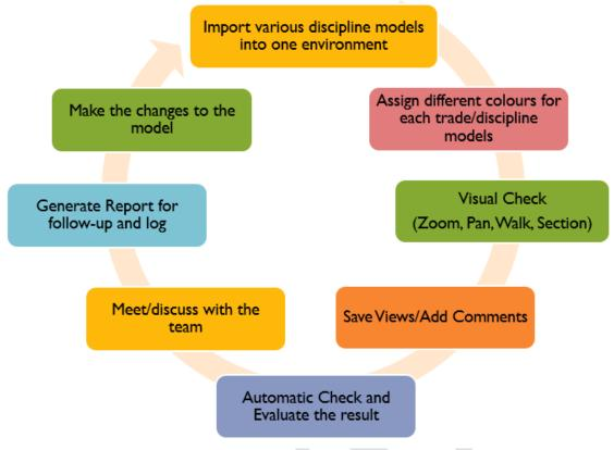
Figure 7: BIM Coordination Step
