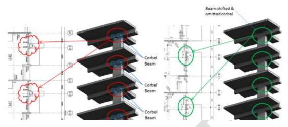
Figure 16: Proposed Design Alternatives – Constructability Checking (Image courtesy of WohHupPte. Ltd)
