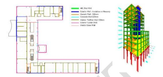
Figure 14: Colour Coding based on Wall Type and Structural Elements – Core Information
