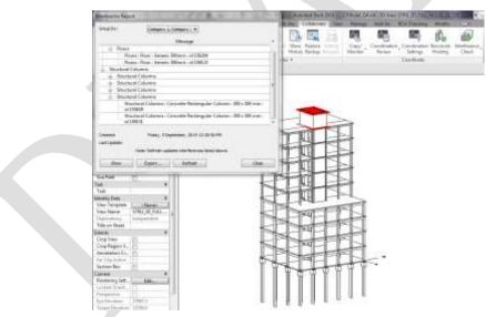
Figure 15: Overlapping and Duplicate Elements
