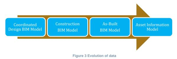
**Coordinated Design BIM Model:** The Design Model is created by the design team that captures the intended design.
