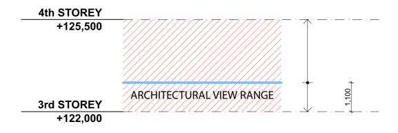
The structural plan views offset the view range downward. Depending on the size
