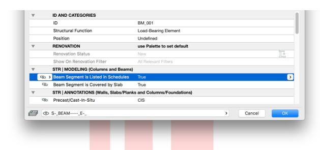
**Note**: Beam schedules focus on the reinforcement and are not listing lengths and volumes. These can be listing by creating separate schedules.
