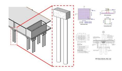
During the construction stage, more detailed information is modelled for the piling. Rebars can also be represented in the model in 3D.
