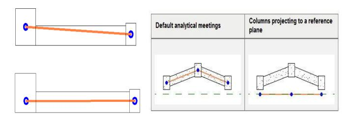
Fig. 17: Beam analytical lines corrected to reflect unsupported length (Image courtesy of CCIT)
