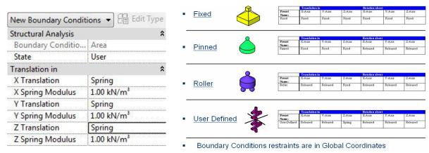
Fig. 12: Soil Spring Supports
