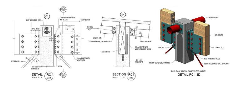
Fig. 30: Structural Steel Connections 2 (Image courtesy of CCIT)
