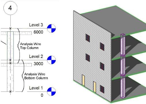
Fig. 14: Columns by Storey (Image courtesy of CSC & CCIT)
