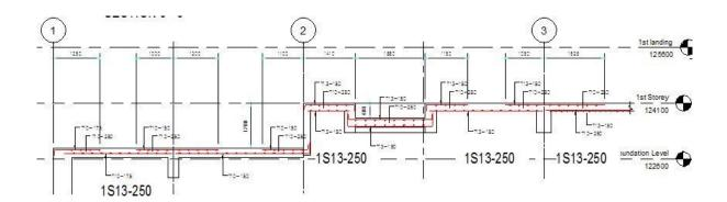
Fig. 23: Structural Slab Detail (Image courtesy of JTC)
