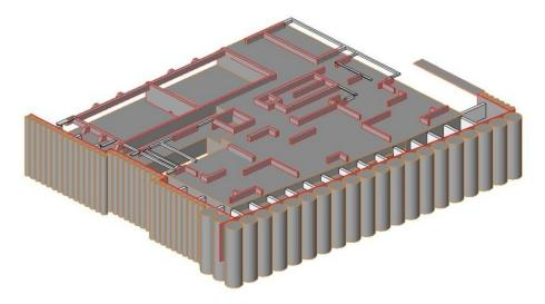
Fig. 3: Continuous Bored Pile (CBP) wall and Mat Foundation (Image courtesy of TYLin)
