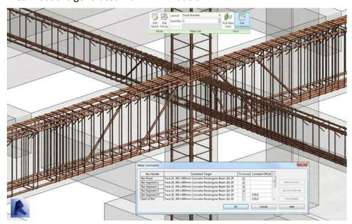
Fig. 24: Structural Beam 3D Rebar (Image courtesy of CCIT)
