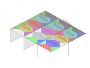
Fig. 15: Floor Slab Load Distribution (Image courtesy of CCIT)
