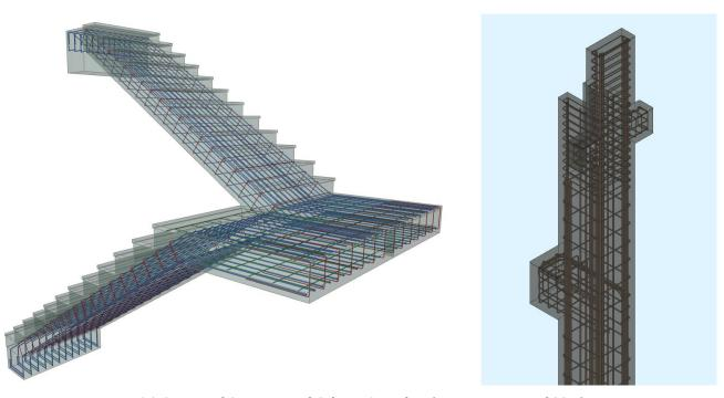
Fig. 25: Structural Staircase and Column 3D Rebar (Image courtesy of CCIT)
