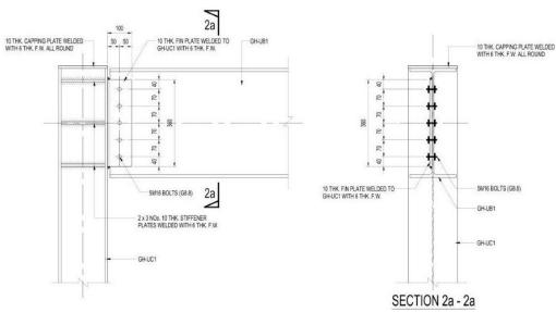
Fig. 28: Structural Steel Connections (Image courtesy of RSP)
