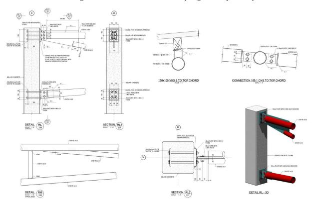
Fig. 31: Structural Steel Connections 3 (Image courtesy of CCIT)
