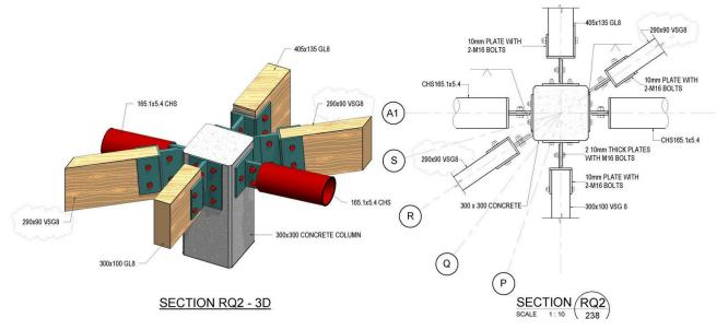
Fig. 29: Structural Steel Connections 1 (Image courtesy of CCIT)
