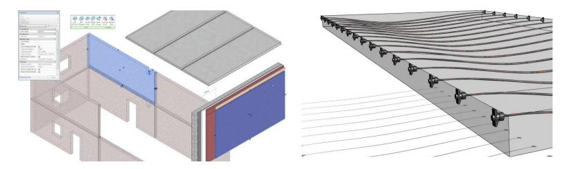
Fig. 26: Revit Precast & Post-Tension Elements (Image courtesy of CCIT)
