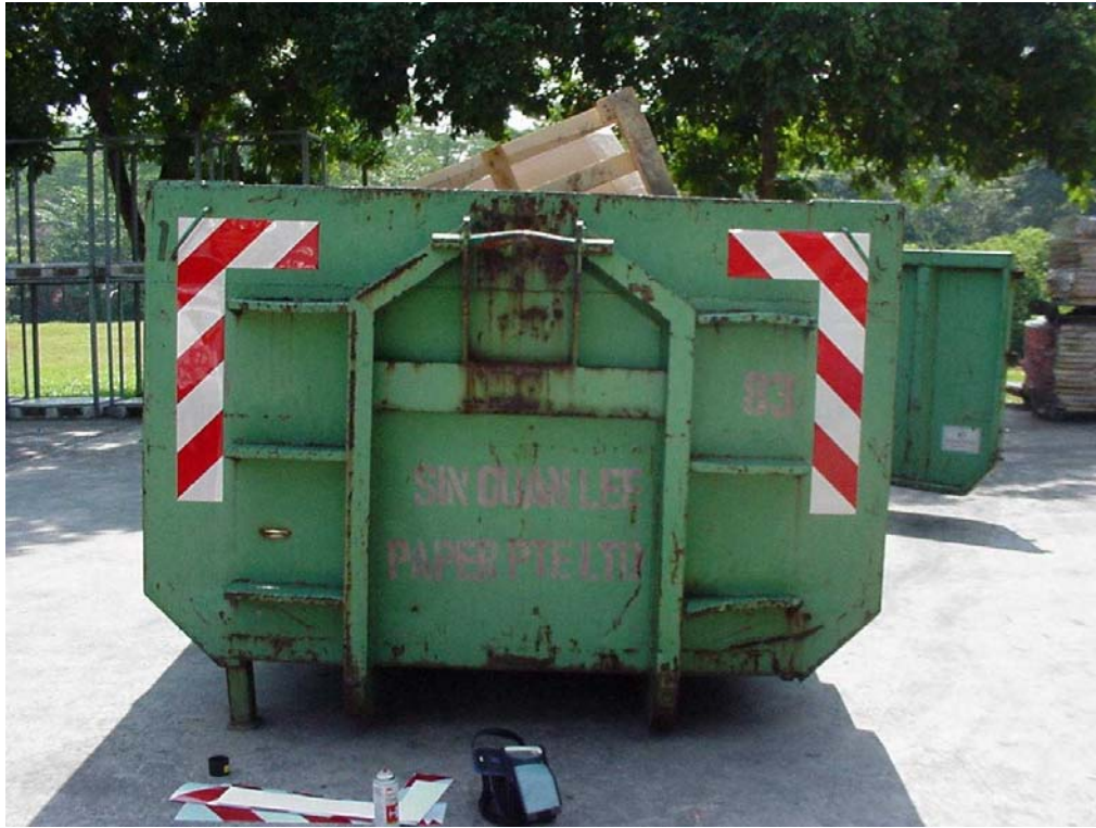
Front View Of Skip Marked With Retroreflective Sheeting
