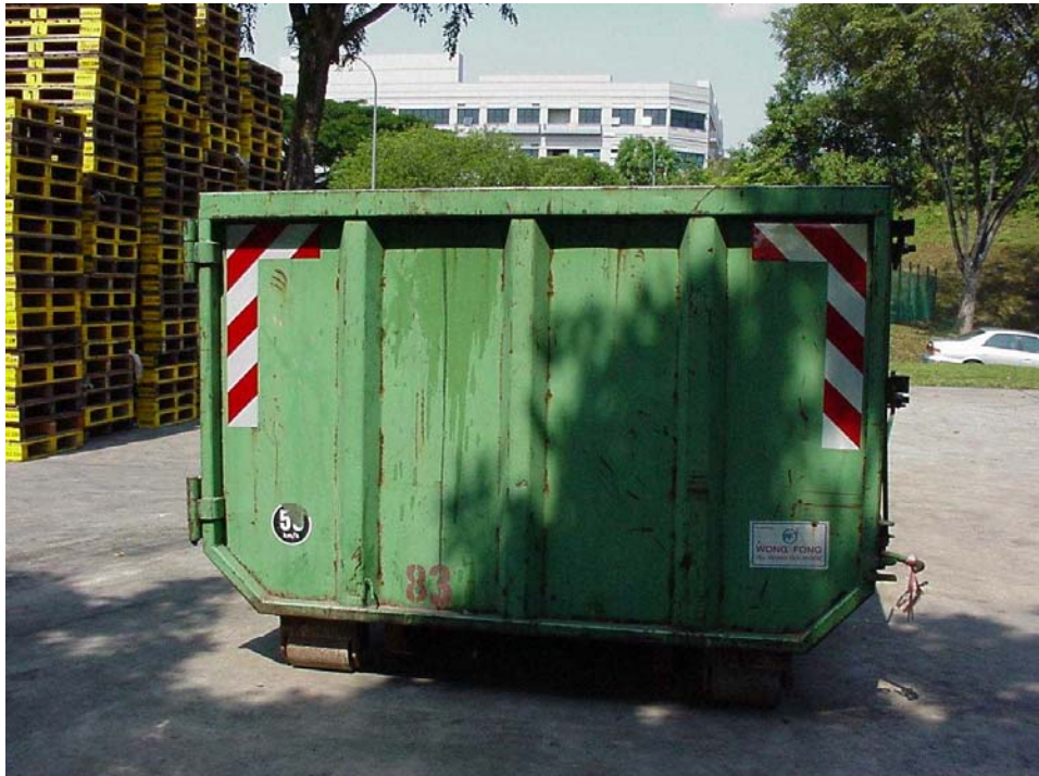
Opposite End Of Skip Marked With Retroreflective Sheeting
