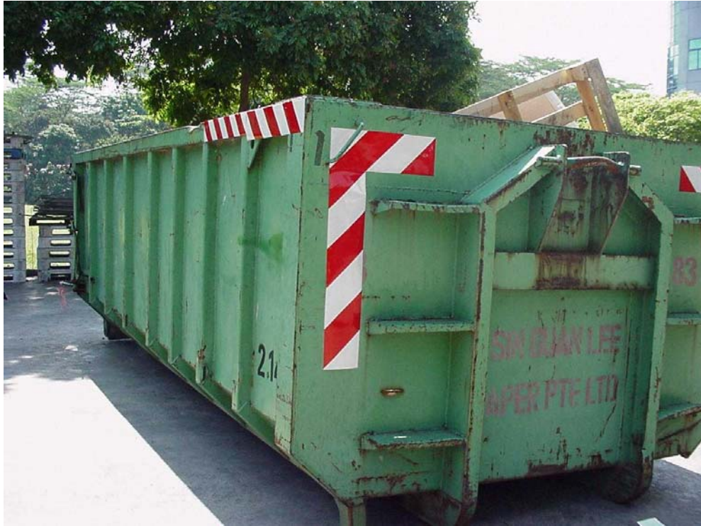
Side View Of Skip With Retroreflective Sheeting
