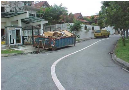
Skip at road bend - "Blind Corner" effect
