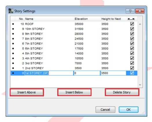
The current template uses the Project Zero as the height reference when displaying elevation dimensions meaning that all elevation heights will be measured from  $\pm 0,00$ .
