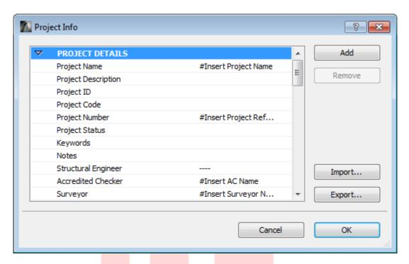
2 Insert all the necessary information of your project in the Project Info dialog and click **OK**. If some fields were not provided with *AutoTexts*, these can be filled out using the **Text tool** from the Toolbox.
