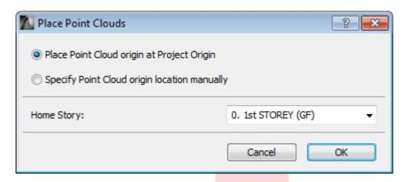
**Note**: the recommended use of imported Point Clouds is referencing only, these objects cannot be used for visualizations.
