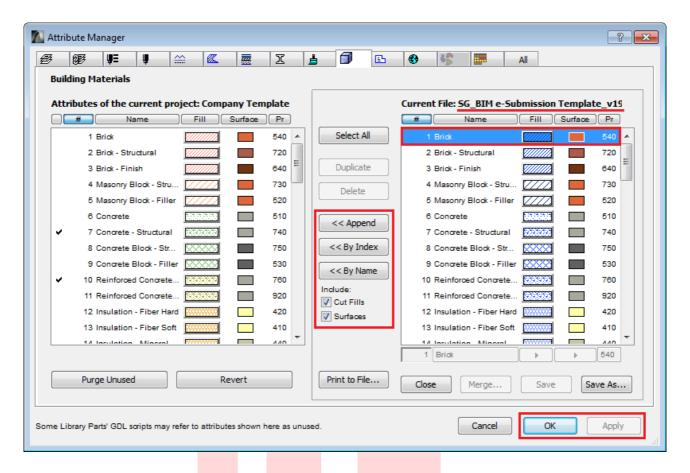
**Note**: The representation of the fills on both sides depends on the actual Pen Set being used by the host file (company template in this example).
