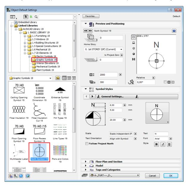
**Note**: the North symbol will only rotate automatically if the orientation is set correctly.
