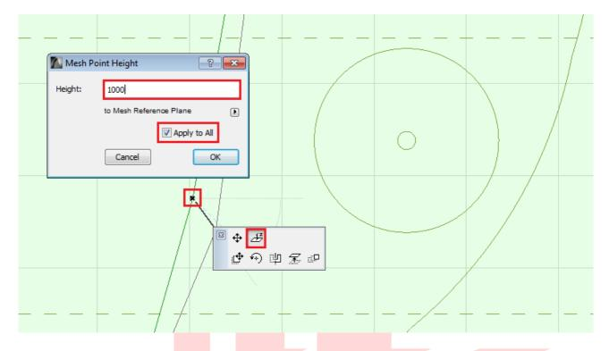
9 As a last step adjust the corner nodes of the mesh (uncheck Apply to All).
