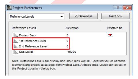
To apply the new reference level, open the **Settings dialog** of an elevation/section viewpoint from the Project Map by right-clicking it and choosing **Section/Elevation Settings**... respectively. On the **Story Levels panel** choose the reference level you set (**Sea Level**). Repeat this with all viewpoints that require the same reference level.
