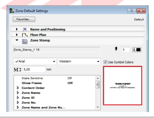
**Note**: To turn on/off the display of the Ventilation Type parameter (or other properties from the Tags and Categories panel) go to **Zone Stamp panel**, **Additional Tags section/1. Row** and change the value to **None** or select one from the available parameters.
