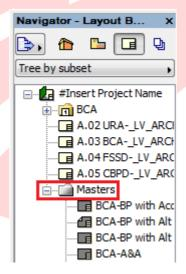
**Note #1**: Avoid changing other parts of the master layout unless you are sure that the AutoText fields (fields containing # marks) are kept intact, otherwise some texts might not appear correctly on the final layouts.
