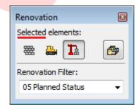
To change all the Renovation Statuses of all the elements (for example change all *New* elements to *Existing* after finishing a phase) use the **Document/Renovation/Reset Renovation Status...** menu command and the upcoming dialog.
