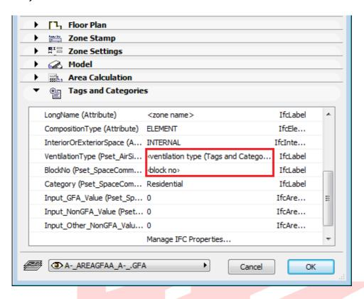
4 Check the appearance of the **Zone Stamp** on the corresponding panel, Zone Name, Measured Area and Ventilation Type should be displayed.
