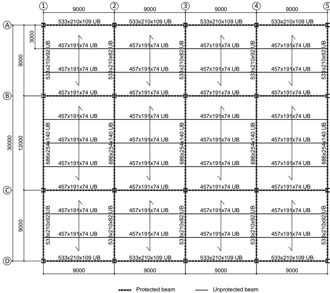
**Fig. B2** Fire-protected and unprotected beams in a typical floor level
