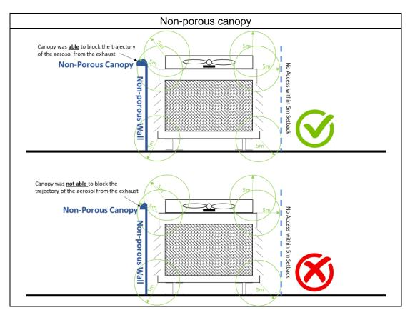
iv. A non-porous wall with the highest edge of the wall at least 5m from the nearest edge of the CT
