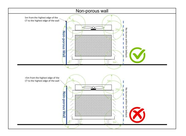
If any air circulating and ventilating inlet, openable window, kitchen exhaust discharge outlet, air handling system or other areas where nutrients conveyed from these systems could assist in the growth of *Legionella* bacteria in the cooling tower system are located within the 5m setback area of the CT, the above-mentioned structural measures of (b)(iii) or (b)(iv) are required to be installed between the CT and the sensitive receptor.
