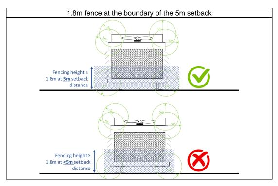
ii. A structure used to elevate the cooling tower such that its base is 6.8m high (5m setback + 1.8m adult height); or
