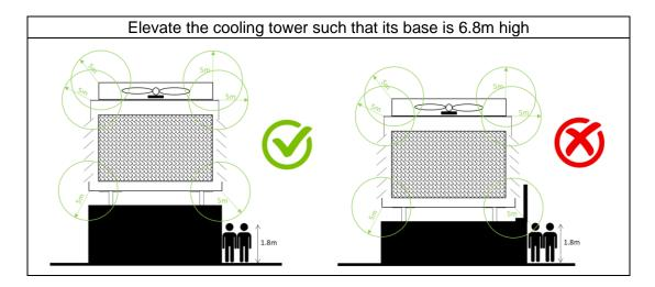
iii. A non-porous wall with a non-porous canopy will need to be built, with the canopy extending to at least 5m (where necessary) from the nearest edge of the CT if the non-porous wall is not of sufficient height to block the 5m plume radius from edge of CT; or
