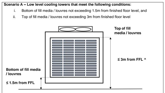
^This allows for the top of fill media/ louvres to be effectively maintained while on FFL or on maintenance platform.
